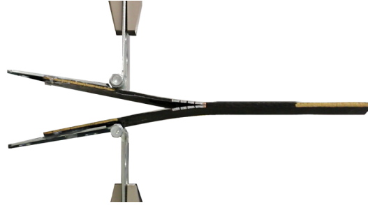
Figure 2.5: DCB test in progress of a carbon fiber laminate with ZnO nanowires
