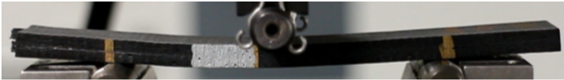
Figure 2.7: ENF test in progress of a carbon fiber laminate with ZnO nanowires
